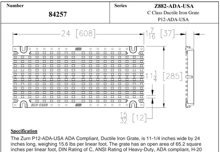
Load Rated. Supplied by Trench Drain Supply.
